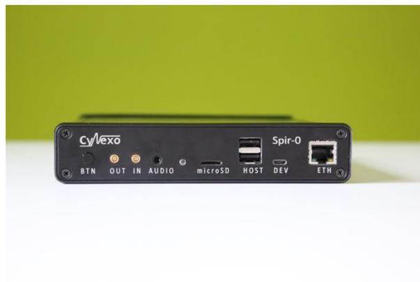
**Spir-0** is an innovative subject breathing activity monitoring tool, extremely compact and simple to use. Its operating principle is based on a fiber optic sensor which makes it compatible with use in MRI, fMRI and EEG environments and applications.
