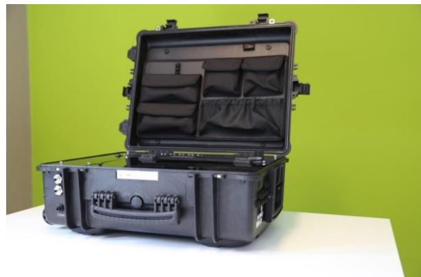
**Sniff-O** is an olfactometer with a brand-new innovative design, feature rich, multi-channel, high-speed, accurate and easily transportable. The number of channels can be customized according to your needs up to a maximum of 13 + 1 channels, while “tailor made” versions can also be created upon request.
